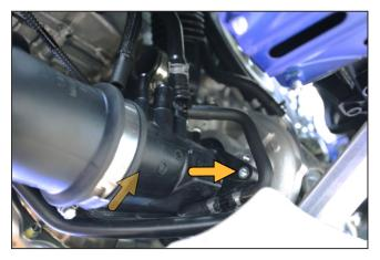
5) Install the Mach 2 in the reverse order of removal i.e. insert the base into the vertical charge pipe first, then push the intake pipe up whilst aligning the recirc outlet.
